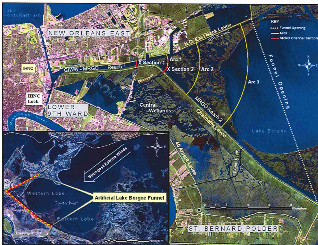
Figure 9. Juxtaposition of hurricane protection levees, marshes, polders, MRGO Reaches 1 and 2 and southern Lake Borgne where surge and waves were generated during passage of Hurricane Katrina (August 29, 2005).
