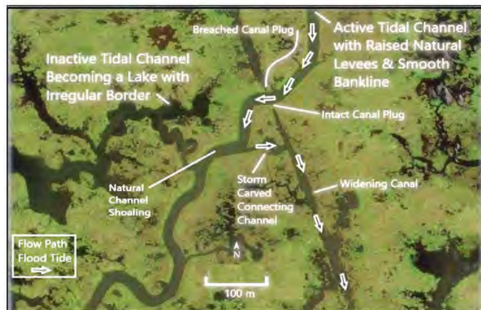
Figure 10. Close-up of western Biloxi Marsh 2 km east of Lake Borgne where a turbid natural tidal channel crosses a canal dredged 15 years earlier. Arrows indicate the flow path on a flood tide. The straight canal captured the discharge of the natural channel when hurricane surge runoff scoured a connecting channel around a canal plug. Abandoned channels/lakes that are cut off from sediment supply appear dark compared to the turbid active tidal channel.
