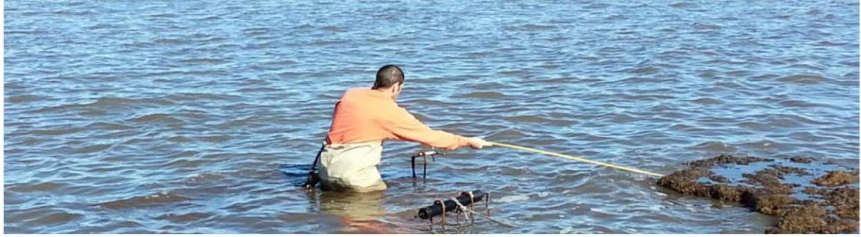
Figure 15 Lower mud scarp on 12/22/2012. During deployment the mud platform extended 1 meter seaward of velocity probe. The photo shows the edge of platform 1.7 m landward of the velocity probe after event 2.
